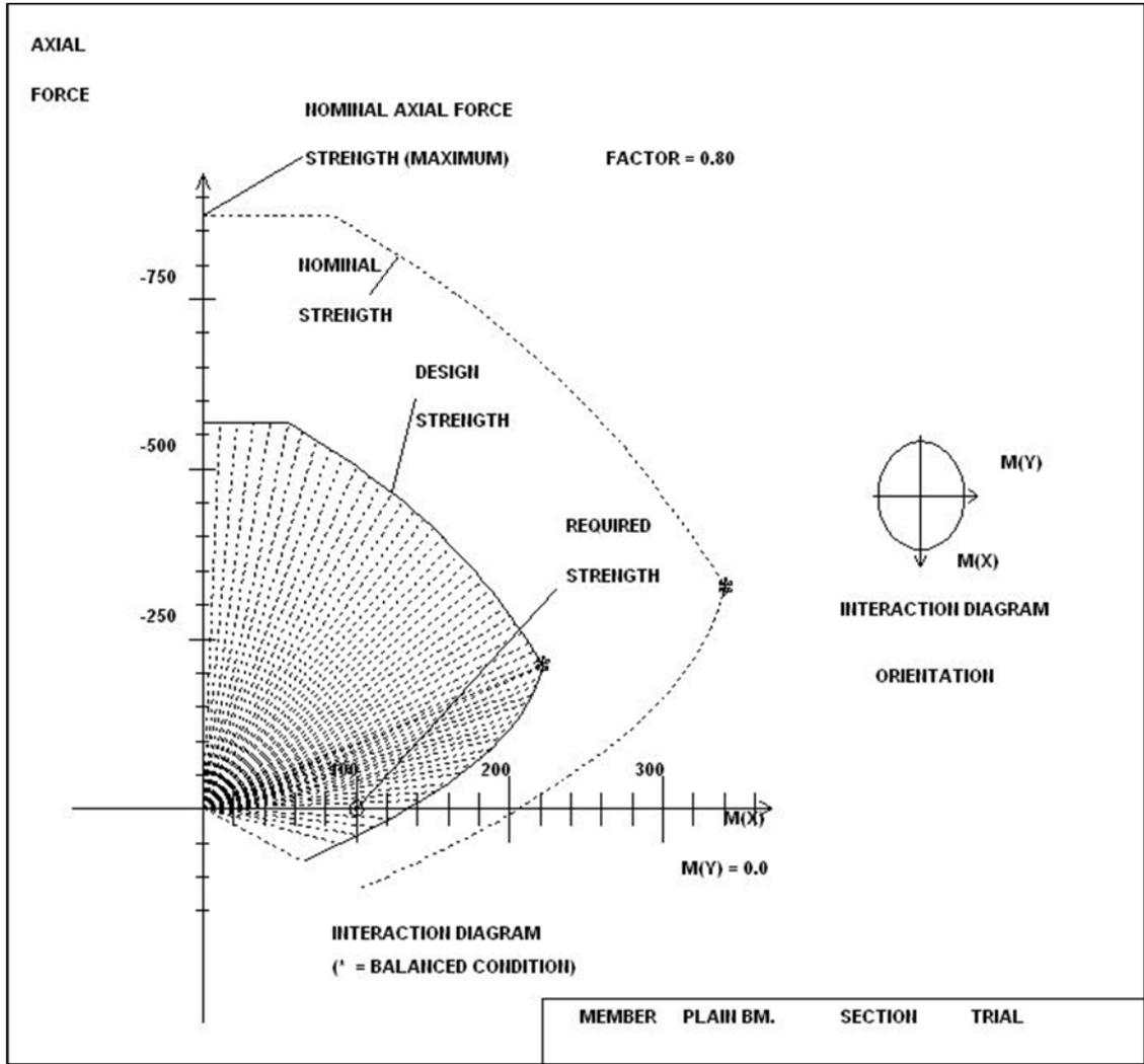
Figure C-8. Interaction diagram produced in the computer program CGSI
