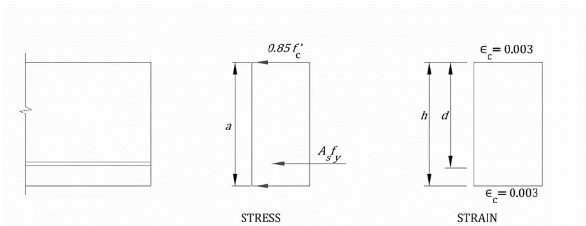
Figure C-5. Stress and strain under maximum axial load
