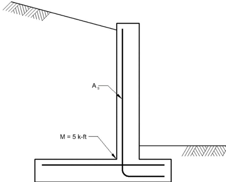
Figure D-3. Retaining wall with moment at the base of stem
