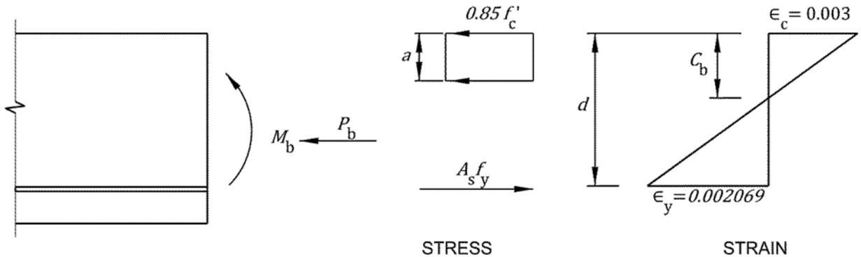
Figure C–6. Stress and strain at balanced point
