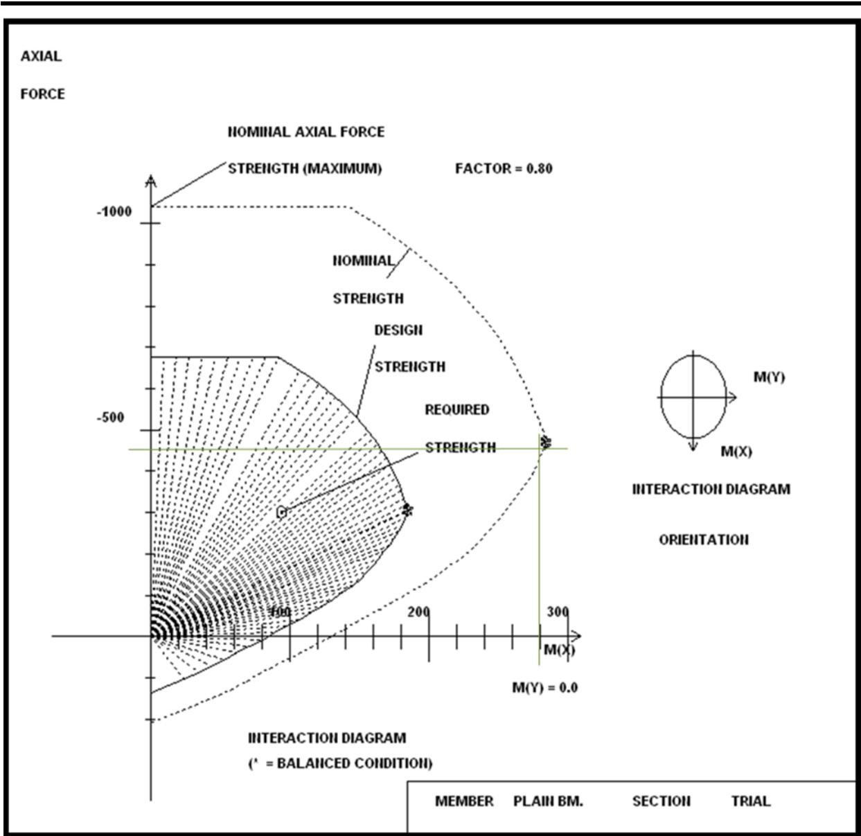
Figure C-13. Nominal flexural strength about the x-axis
