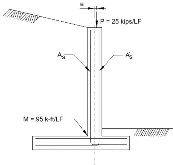
Figure D-4. Retaining wall with moment at the base of stem plus axial load
