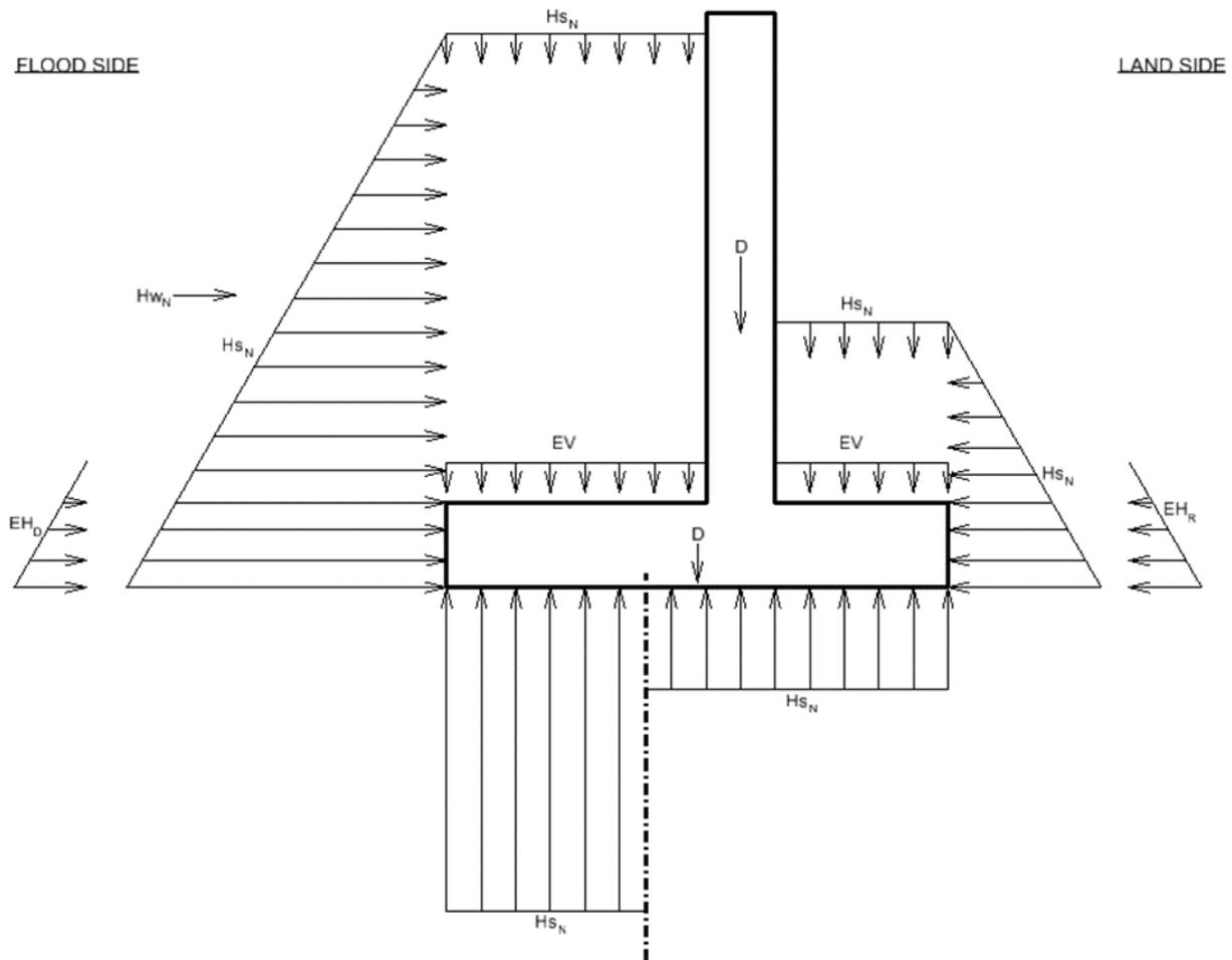
**Figure D-5. Coastal floodwall with Load Case 1.1 loads (Table D-3a)**
