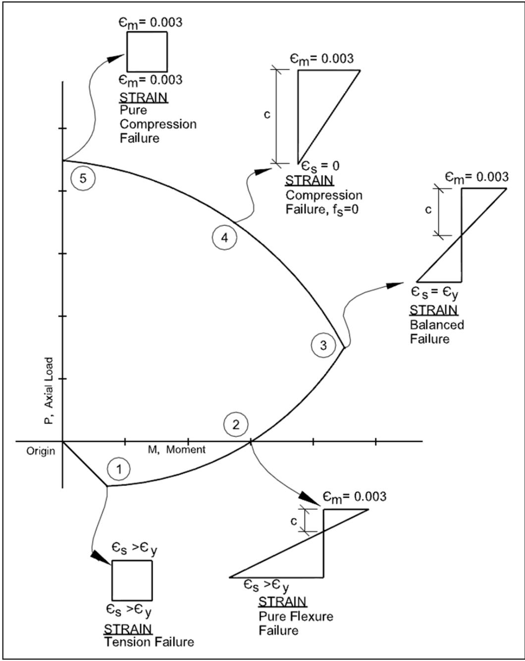
Figure 4-2. Interaction diagram illustrating strain conditions
