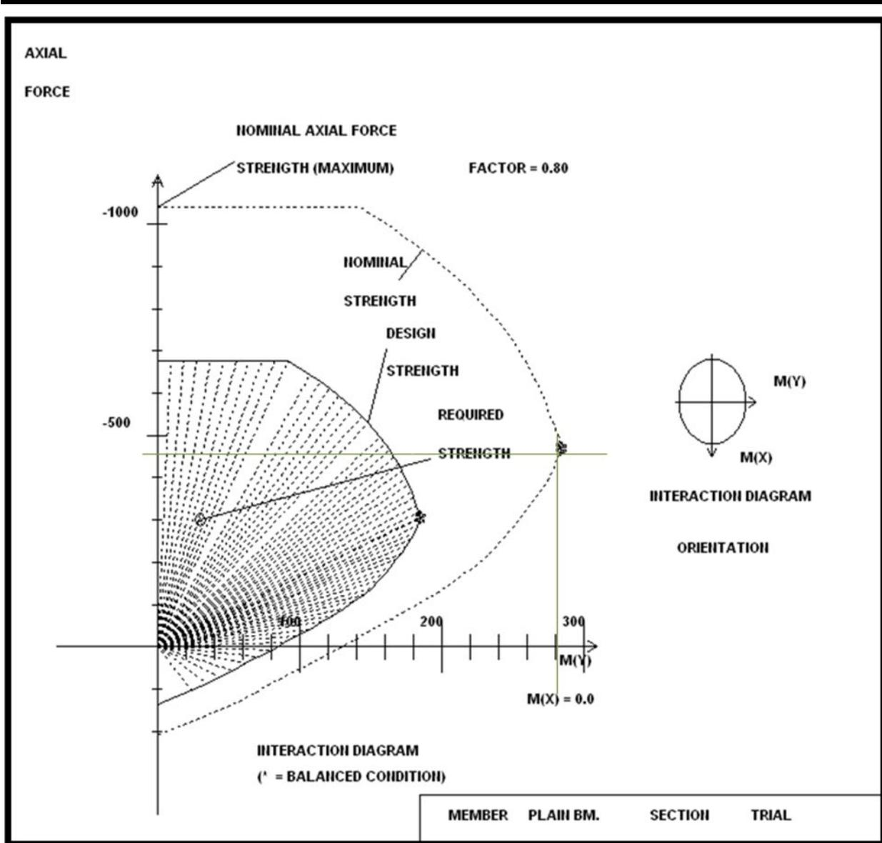
Figure C-14. Nominal flexural strength about the y-axis
