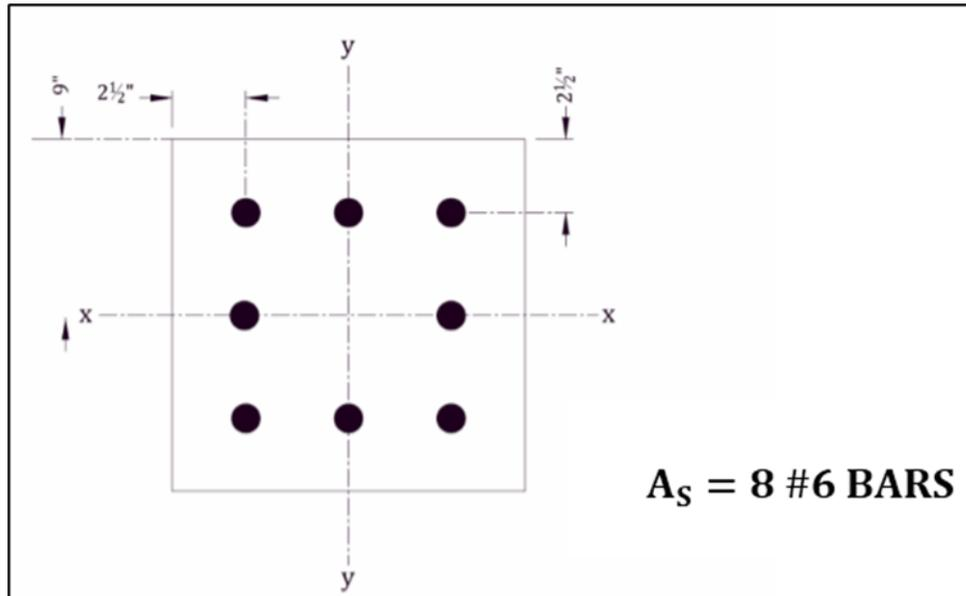
**Figure C-9. Cross section of column with 8 #6 bars**
