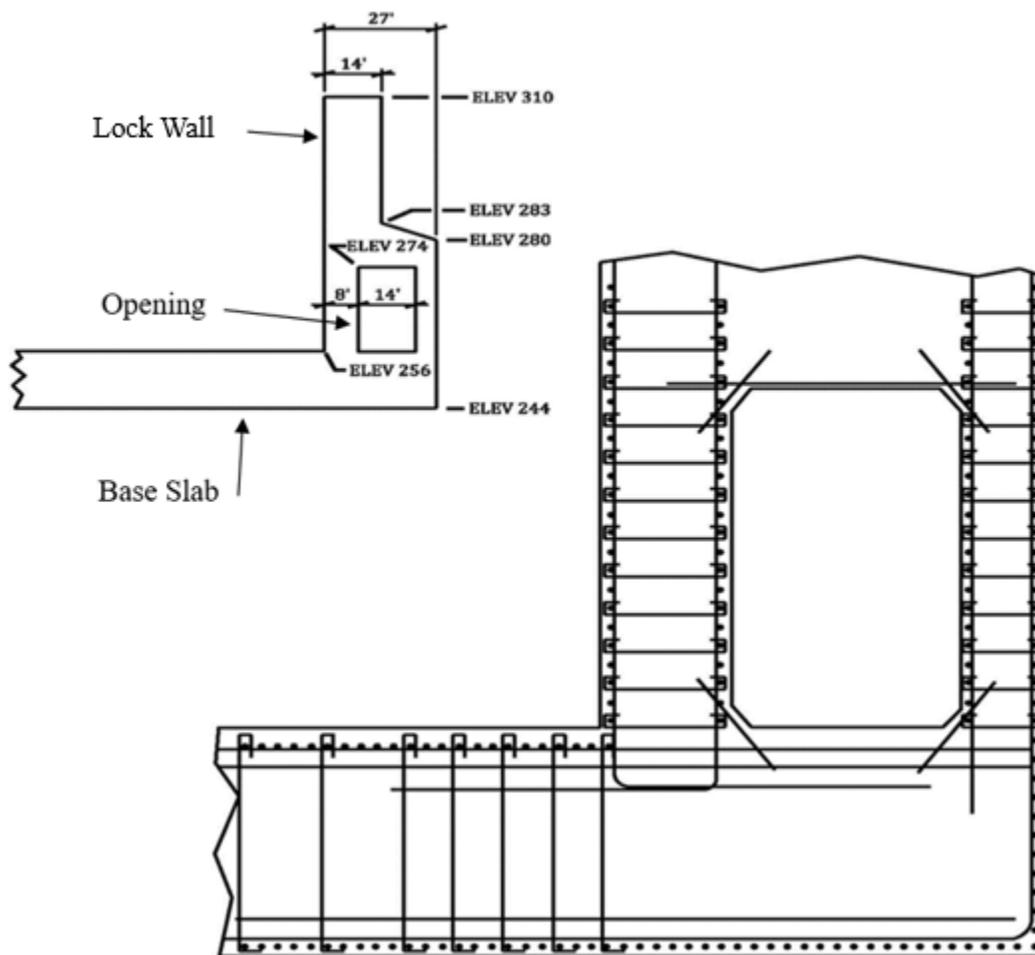
Figure 2–2. Typical seismic reinforcement details – Olmsted Lock and Dam
