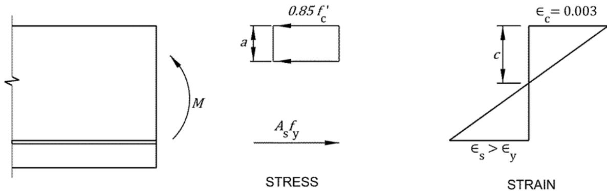
Figure C-4. Stress and strain under pure flexure
