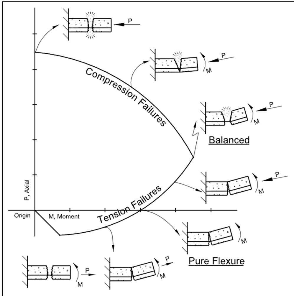
Figure 4–1. Interaction diagram with illustrated failure modes
